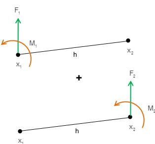
Therefore, we simply need to add  $F_1$  and  $M_1$  in the first 2 rows of force vectors ( $F_2$  and  $M_2$  in the last 2 rows which is same as Example 7).
