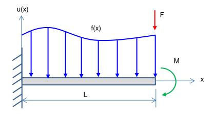
The equation of the above cantilever beam by Euler-Bernoulli's beam theorem (skipping the explanation of this theory) will be **4**<sup>th</sup> **order differential equation**.
